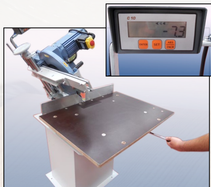
Vertical tilt from front of machine with digital angle display.
