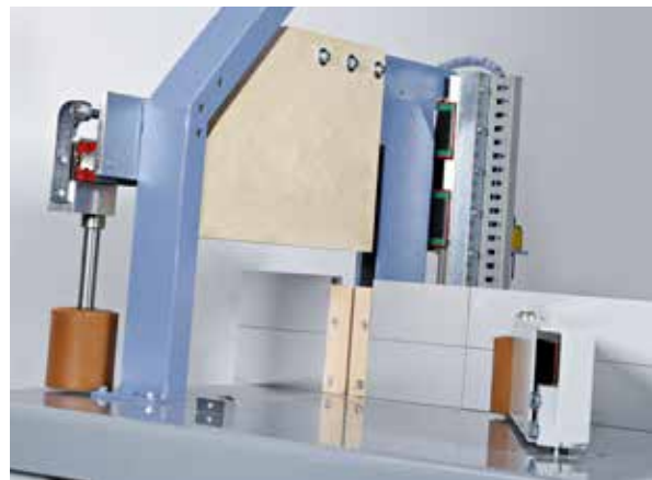
Detail of the upper workpiece clamp.
