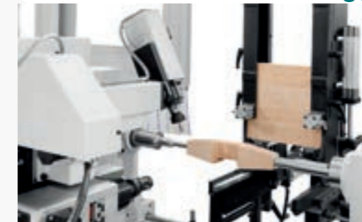
Detail of machining two sofa legs at the same time with tilted vertical router head.
