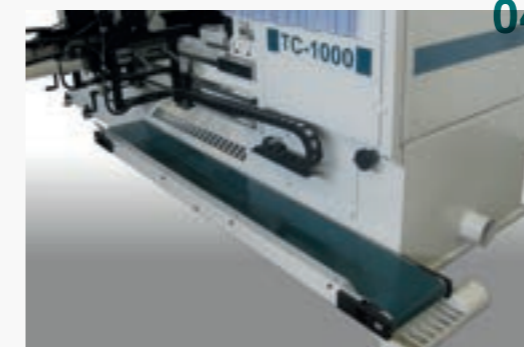
Optional equipment: Transfer exit belt to eject the finished parts.
