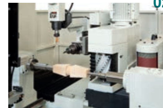
Detail of machining two sofa legs at the same time with straight vertical router head.
