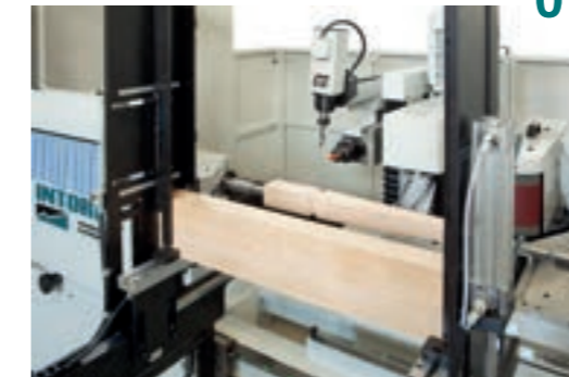
Standard machine: frontal hopper feed loader, horizontal router head, vertical (tilt) router head, shaping and sanding unit.
