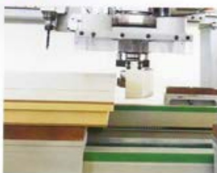
Squadratura porta Countouring with C Axis and dust deflector
