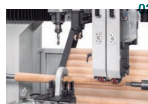
Two CNC copiers for sanding working simultaneously with the turning process.
